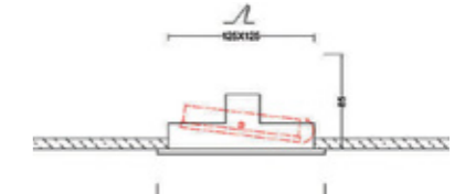
Cutting Hole 125 mm x 125 mm
