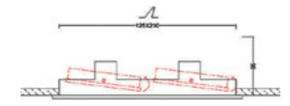
Cutting Hole 125 mm x 210 mm
