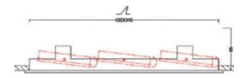
Cutting Hole 125 mm x 315 mm
