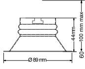
Cutting hole diameter 78 mm
